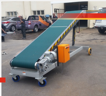
Truck Loader & Conveyor System
